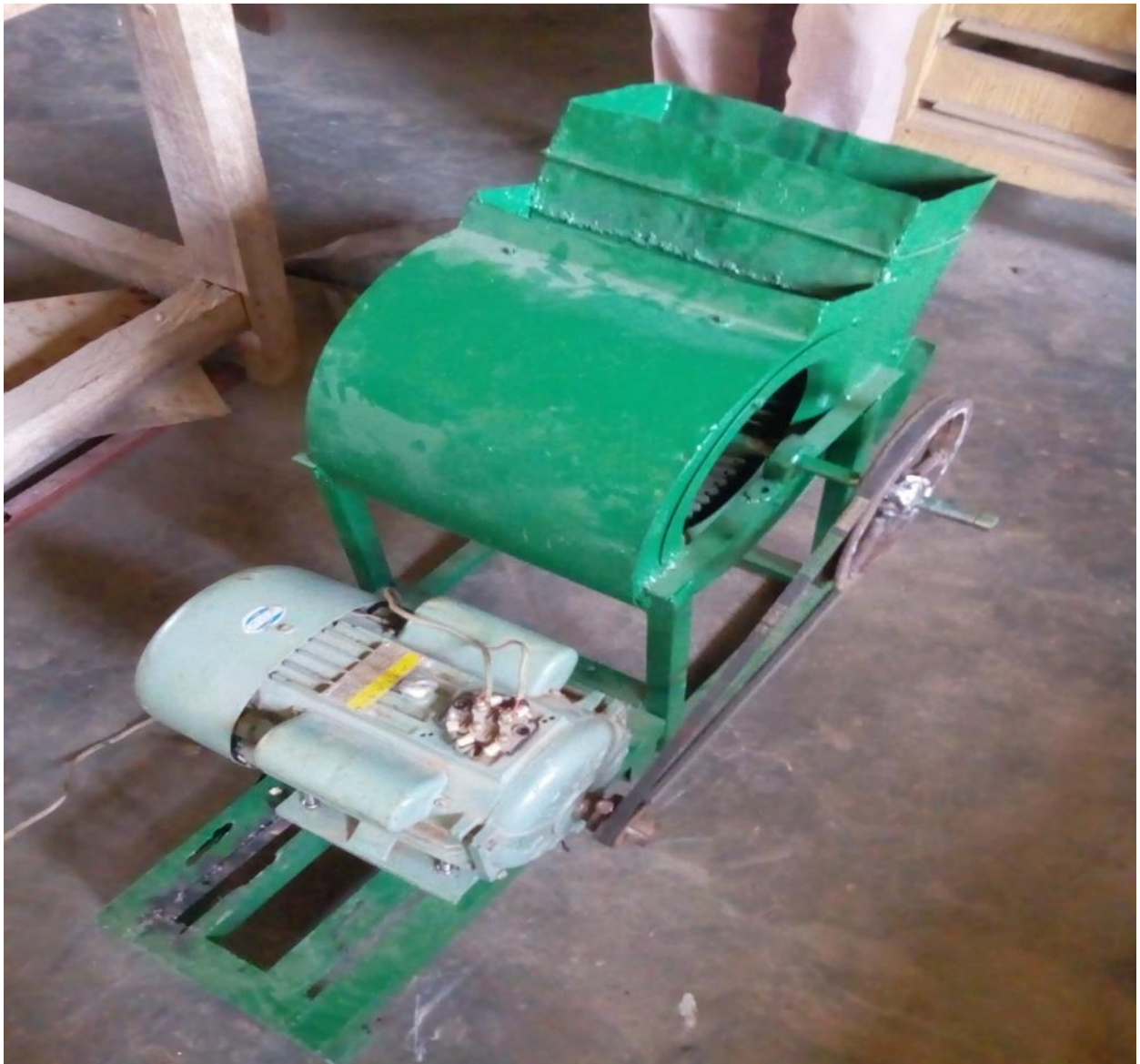
Plate 2 Pictorial view of the fabricated centrifugal fan.
